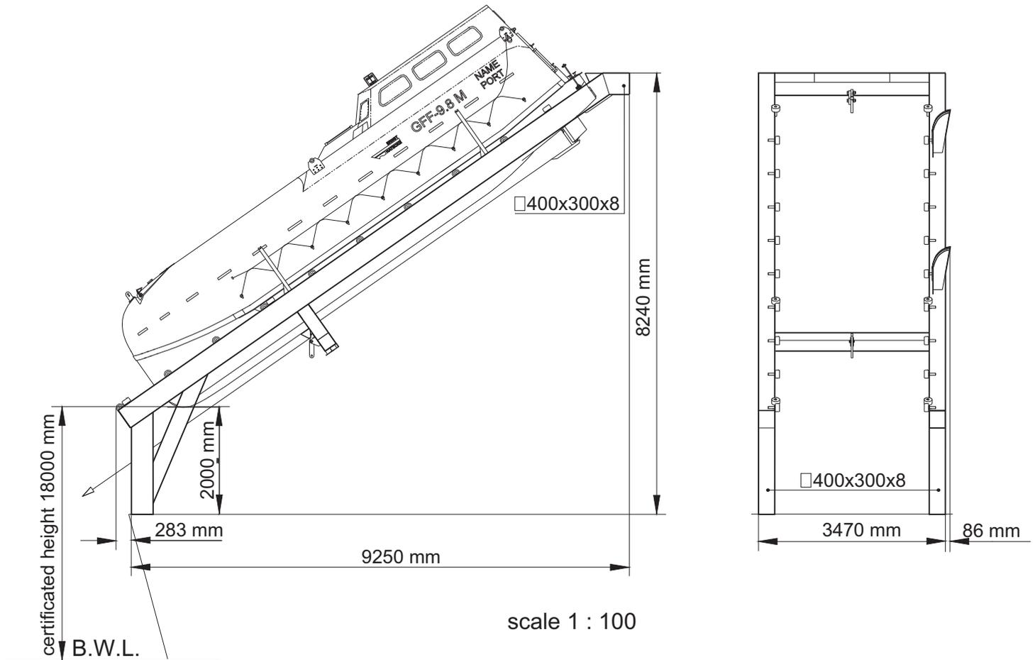
Length adjustment of horizontal and vertical supports in accordance with shipyards request.
